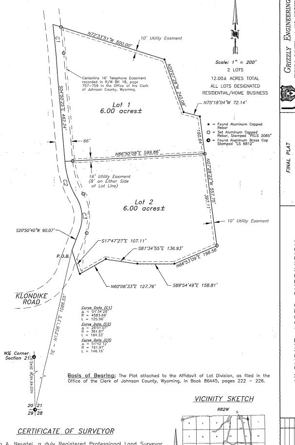
I, Keith A. Neustel, a duly Registered Professional Land Surveyor in the State of Wyoming do hereby certify that this Plat of the KLONDIKE ACRES SUBDIVISION is based on existing deeds of record, existing plats of record and on the results of a field survey conducted under my direction as a Registered Professional Land Surveyor.
