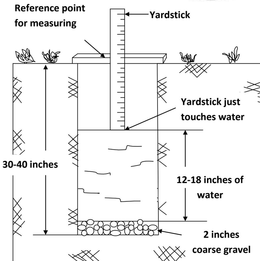
Side view of a typical percolation test. Yardstick is lowered to the surface of the water after each time interval. Time interval and measurement are noted and recorded. When measuring use the reference point as a guide.
